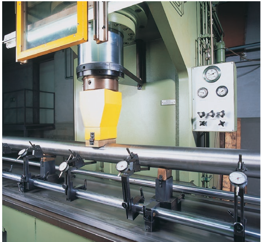
Straightening of a shaft Ø 140 mm
