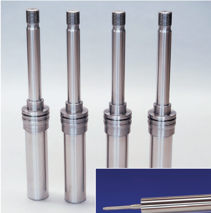
Pistons Turned part with roller- burnished radii, grinded and hard chrome plated
