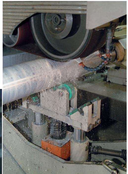
Belt grinding assembly and supporting steady rest
