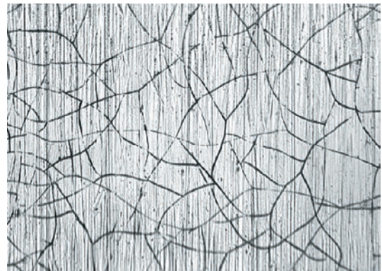
Surface image Crack structure double-chrome layer
