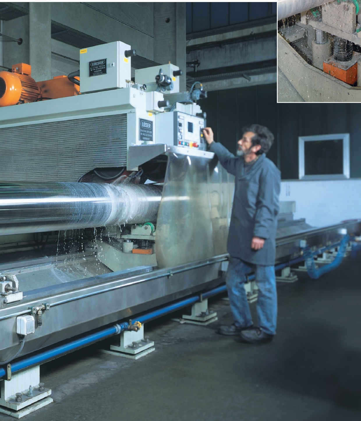
Belt grinding assembly and supporting steady rest
