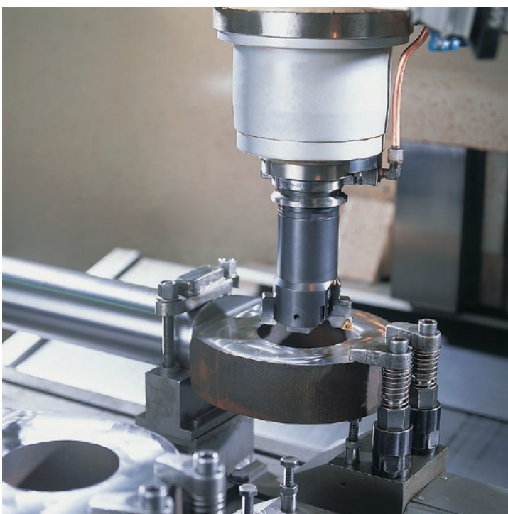
Processing piston rod eye
