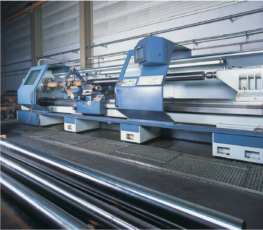
Production of long turned parts
