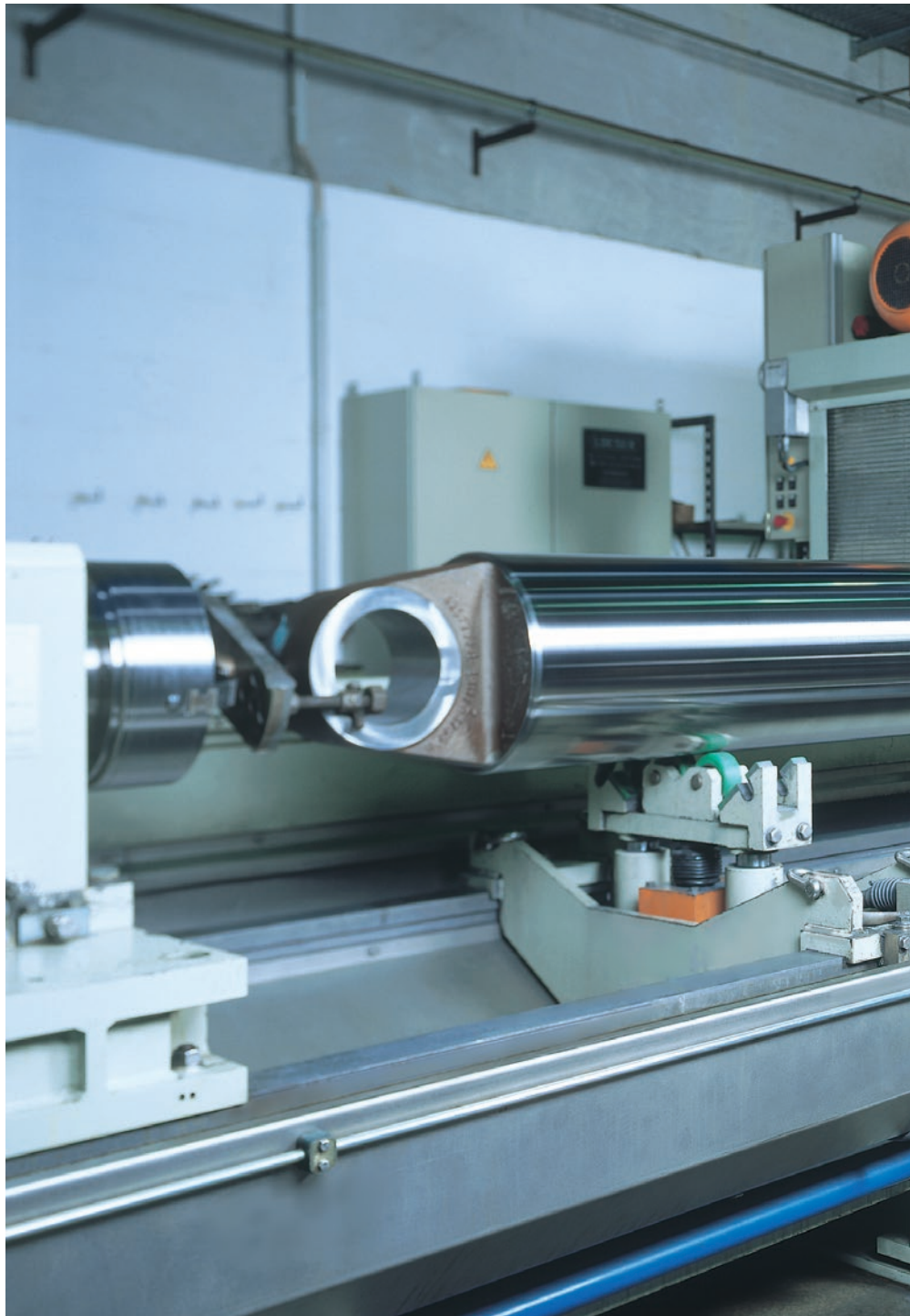
Belt grinding of a piston rod Dimensions Ø 400 x 4,800 mm
